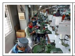
Linking machines were installed near the wall without confirming 0.75m space
