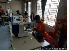
Bartack machine were installed near the wall without confirming 0.75m space
