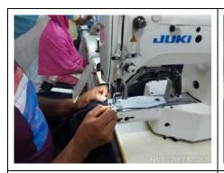
Bartack machine did not have any needle guard NC Picture No. 04
