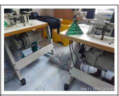
Lower pulley guards were found not fully covered with overlock machines
